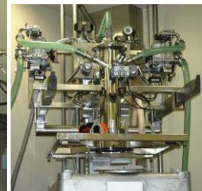
Figures: Left/below: Central transfer- and dosing station including a PTS with 3 product entries fixed on a frame which can be lowered on a container positioned on a scale.
