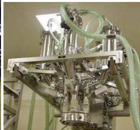
Figures: left: central transfer- and dosing station including 5 PTS connected to a container positioned on a scale. below: Central transfer and dosing station fixed on the support frame.
